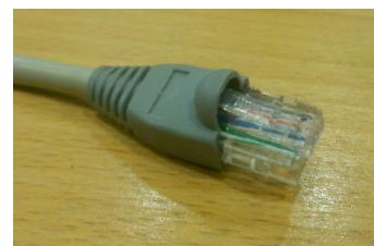
(obr. 3 - Kabel RJ45)
